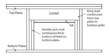
Openings greater than 10 feet in width, minimum 2 Jack Studs
